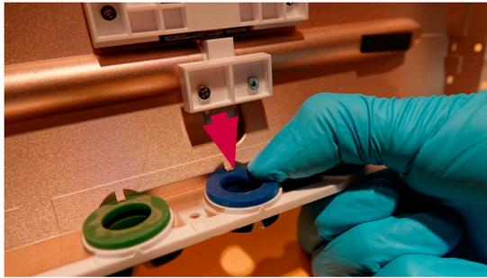
Figure 20 Remove the damaged colour ring
