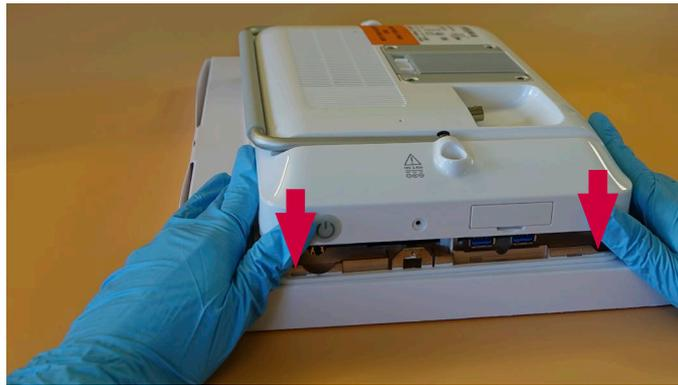
*Figure 31 Place the back casing, continued*
