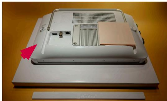
*Figure 8 Place the displaying unit facing down*
