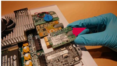
Figure 17 Remove the VDI board
