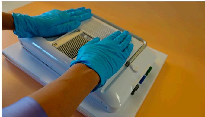
*Figure 32 Press down on the back casing until it clicks in place*
