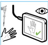
Ensure that a live image is displayed on the monitor by pointing the distal end of the visualisation device at an object.
