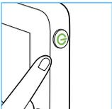
Press the power button to turn on the monitor. It takes approximately 20 seconds for the system to fully load, however a live image can be displayed after just a few seconds.
