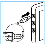
Connect the Ambu visualisation device to the aView 2 Advance monitor, making sure that the arrow on the cable connector lines up with the white triangle on the connection port.
